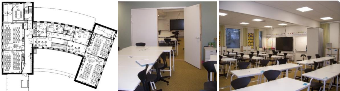
Floorplan of first floor of the renovated building (left). In the original building, double doors connect teaching spaces (centre) while sliding walls are used in the new wing (right).
