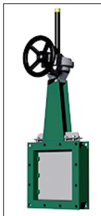
Figure 2.2: An illustration of a manually operated penstock type gate with a valve
