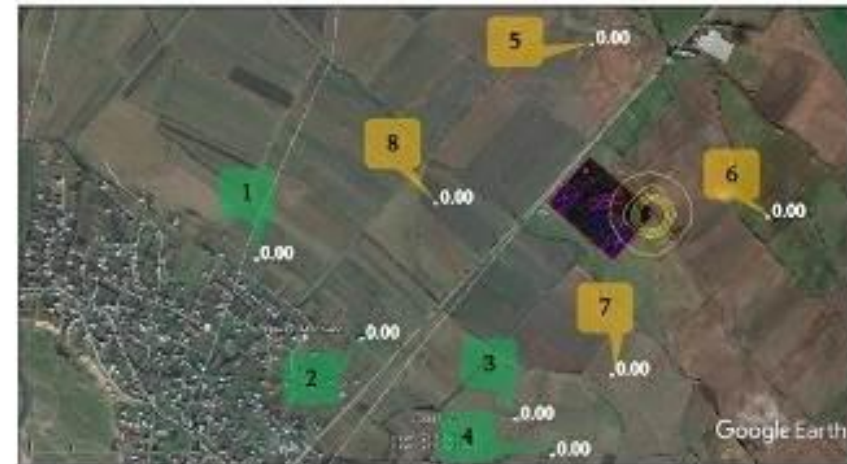
Maximum concentration of sulphur hydrogen (code 333) at control points (nos. 1-4), at the nearest settlements and at the border of 500-m rated zone (nos. 5-8)
