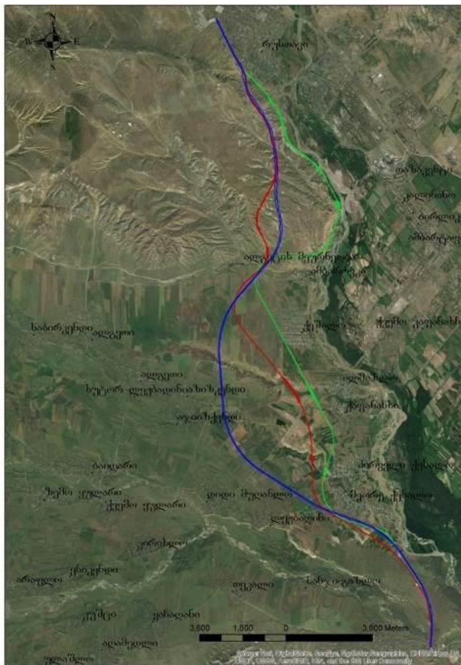
Figure 3.1.2.1. Alternatives of the highway alignment
