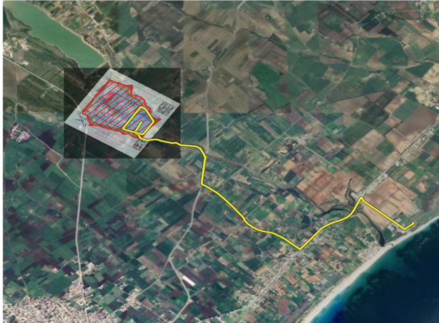
Figure 12 : Converter station area and HVAC cable route
