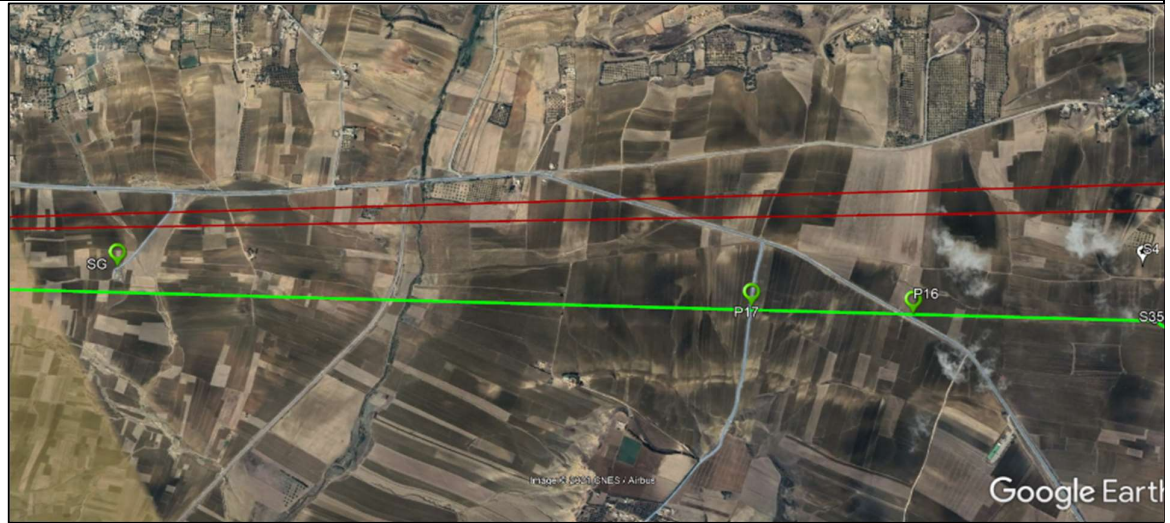
Figure 32 : Presence of a gas pipeline near the area proposed for the OHL line at P16 and P17
