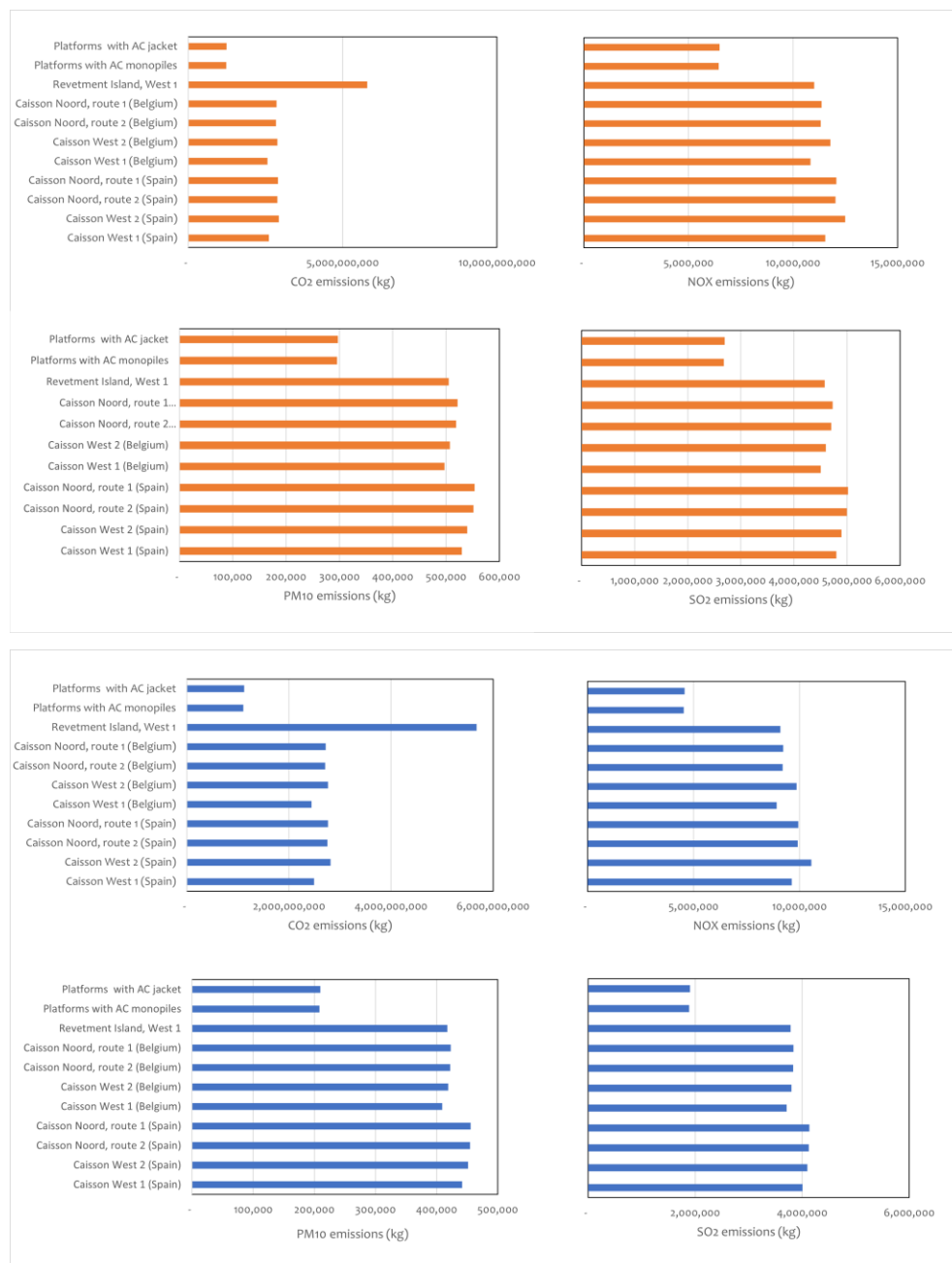
Figure 6-2 : Total emissions for four pollutants for all scenario's for the long term scenario 50 years: cable pre-trenched scenario on top (orange) and cable pre-ploughing bottom (blue).
