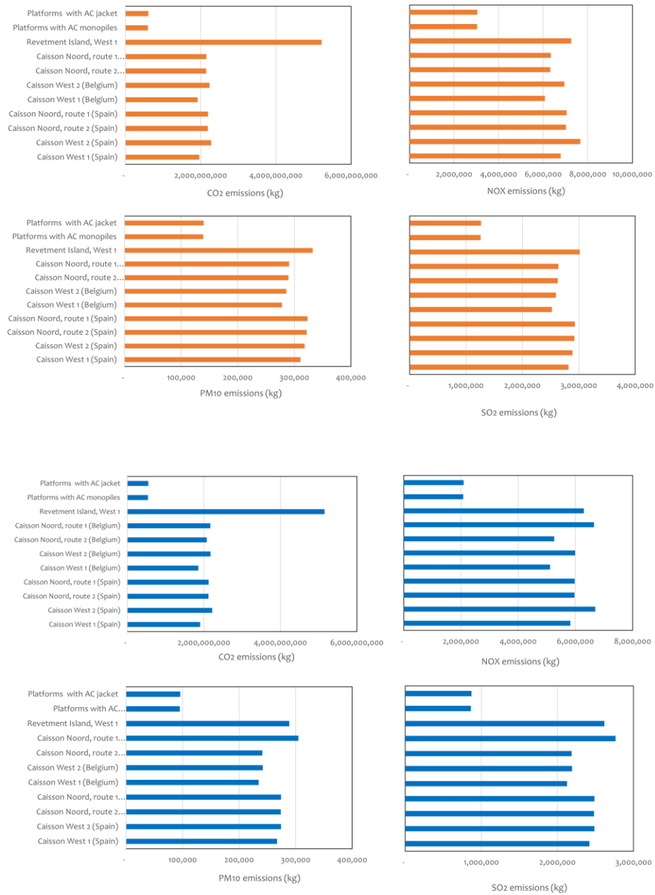
Figure 6-1 : Total emissions for four pollutants for all scenario's for the permit duration of 20 years: cable pre-trenched scenario on top (orange) and cable pre-ploughing bottom (blue).
